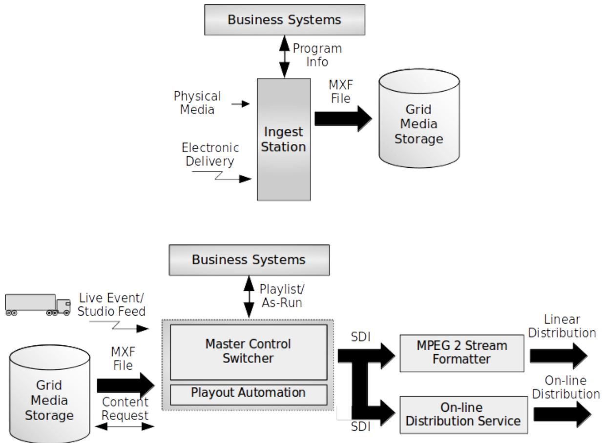
**Figure 5. Traditional SDI/File-based Master Control Facility**
