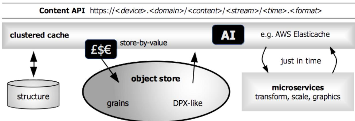
**Figure 11. A Common Content API Provides A Uniform, Open Interface To Essence**
